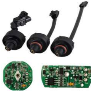
Water Level Sensor
